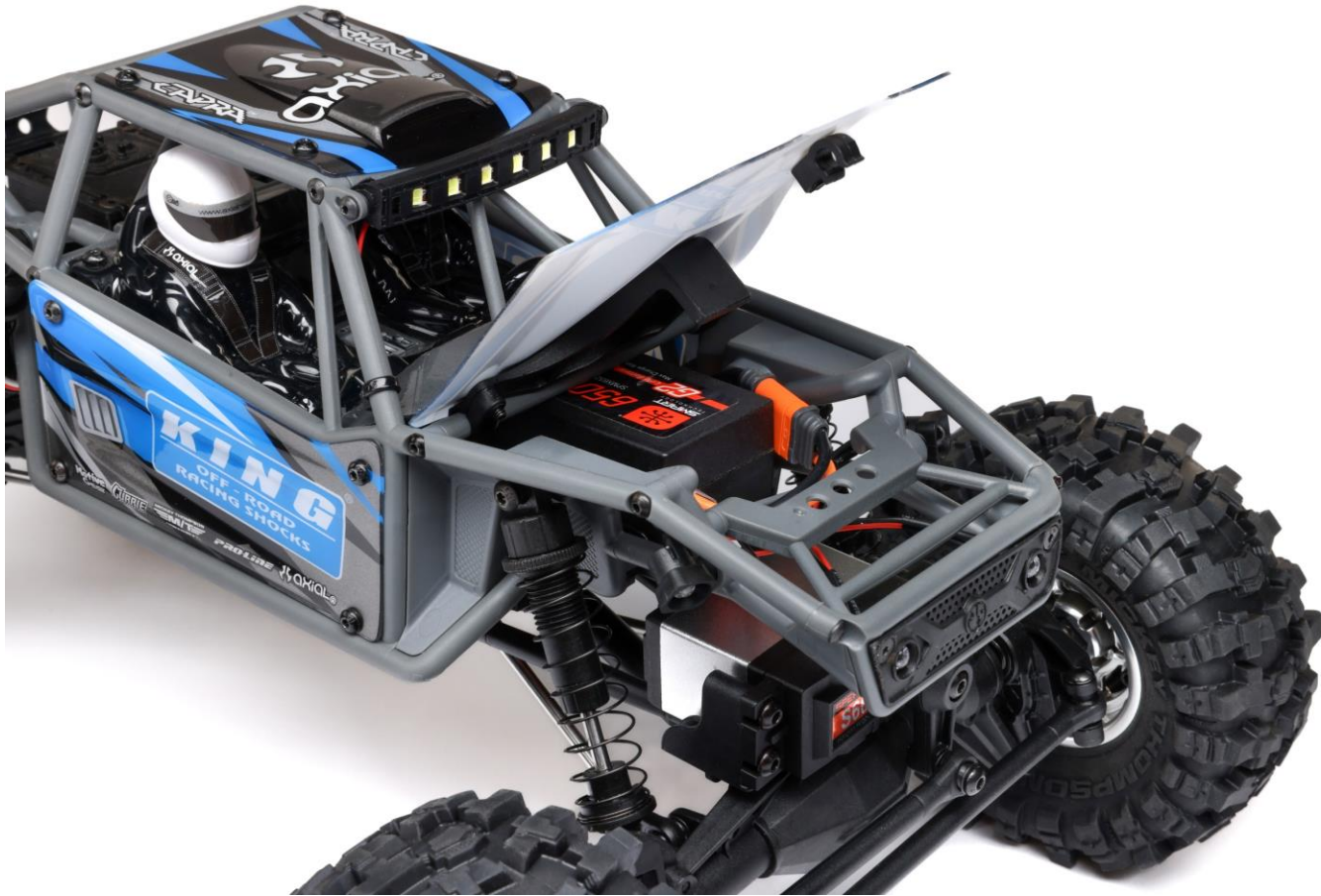
Included Spektrum LiPo battery mounts under hood panel.
